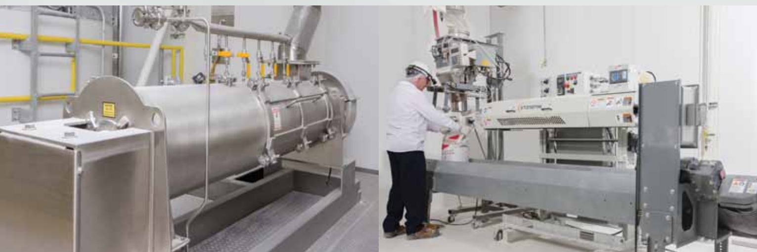
At Huber's state-of-the-art Quincy, Illinois, operation, HuberCal ® pure and natural calcium carbonate is granulated to exacting specifications (photo above left). HuberCal products are bagged and prepared for shipment (photo above right).
